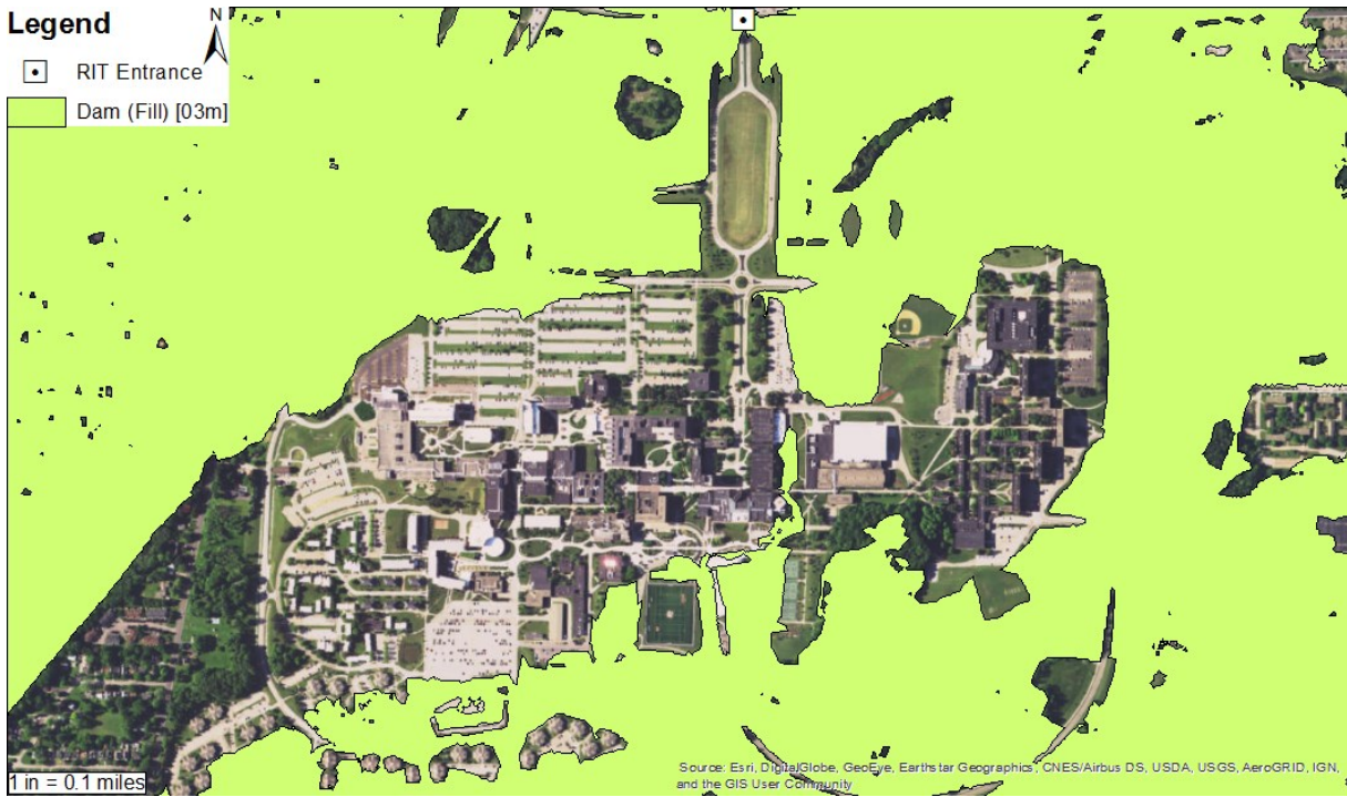
Figure 30 - Dam (Fill) [03m]. This figure demonstrates the 3m cell size data's ability to closely follow features in the built environment nearly as well as the 2m cell size data, preserving fine details such as property boundaries.
