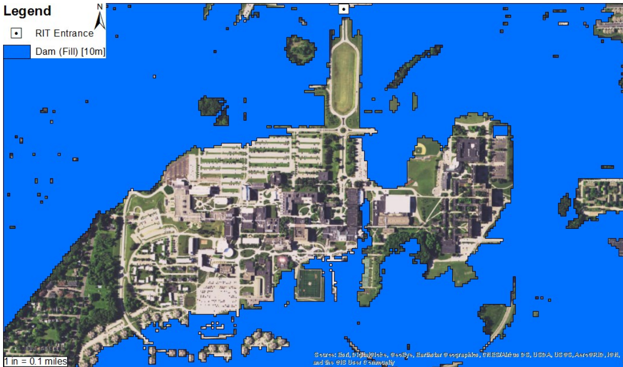
Figure 32 - Dam (Fill) [10m]. This figure demonstrates the 10m cell size data becoming noticeably abstracted from the built environment, featuring clean straight lines where they're not present.
