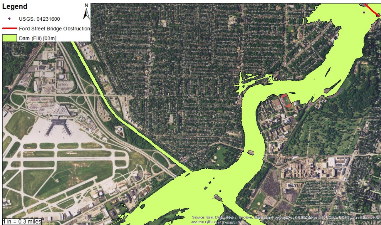
Figure 23 - Dam (Fill) [03m]. This figure demonstrates the fine granularity of the 3m cell size flood extent generated by the FEG.
