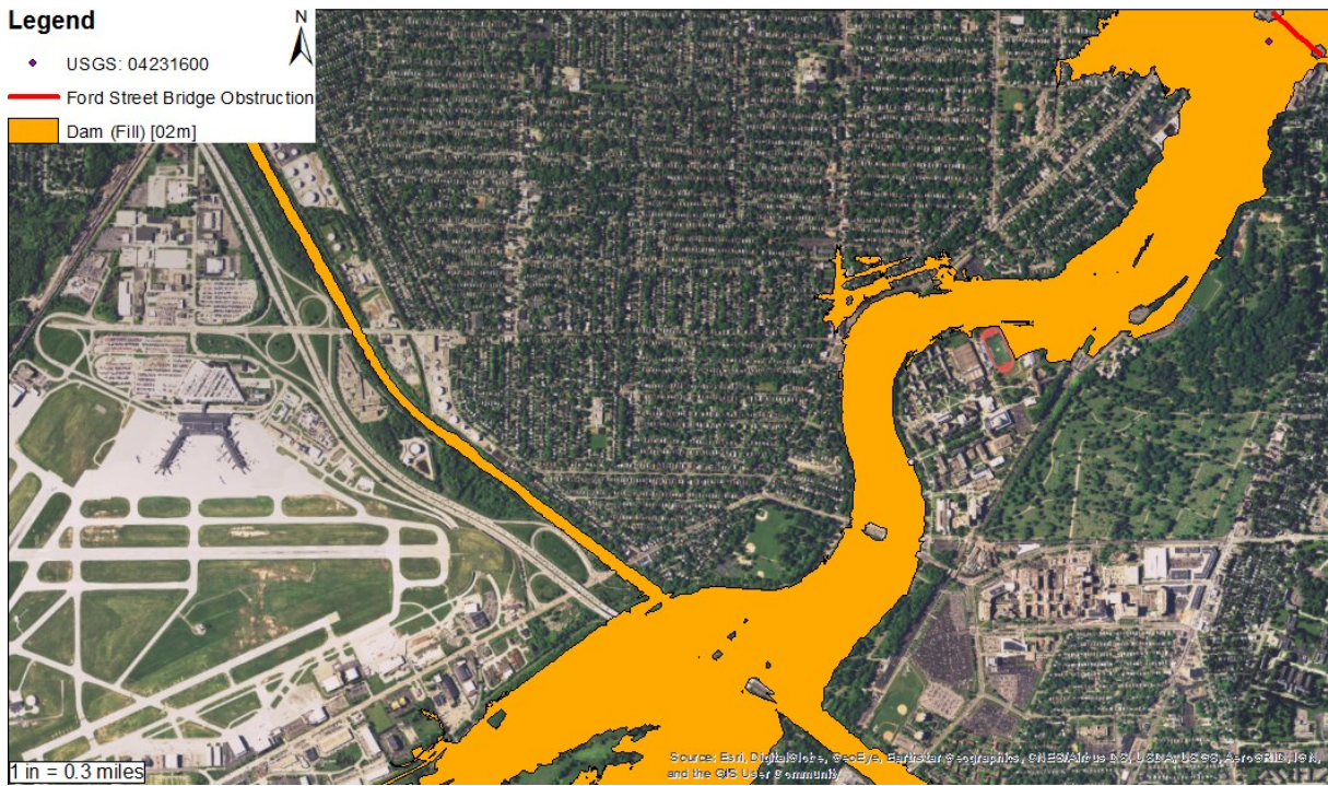
Figure 22 - Dam (Fill) [02m]. This figure demonstrates the fine granularity of the 2m cell size flood extent generated by the FEG.
