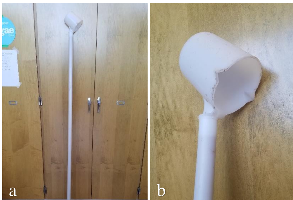
Figure S-1. 500 mL graduated water dipper; a) 60-ft long dipper, b) 500 mL cup.
