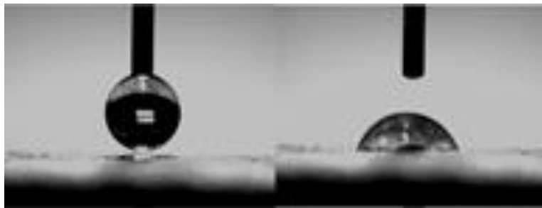
Figure 43 Wicking Rate Calculated by Rate of Decrease in Contact Angle
