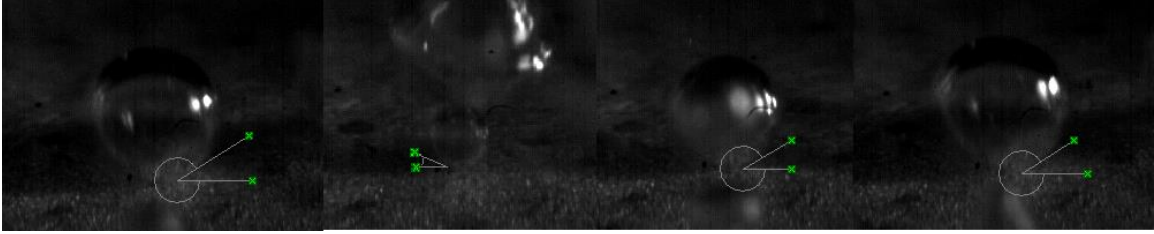
Figure 41 Dynamic Receding Contact Angle Measurement for SP_213
