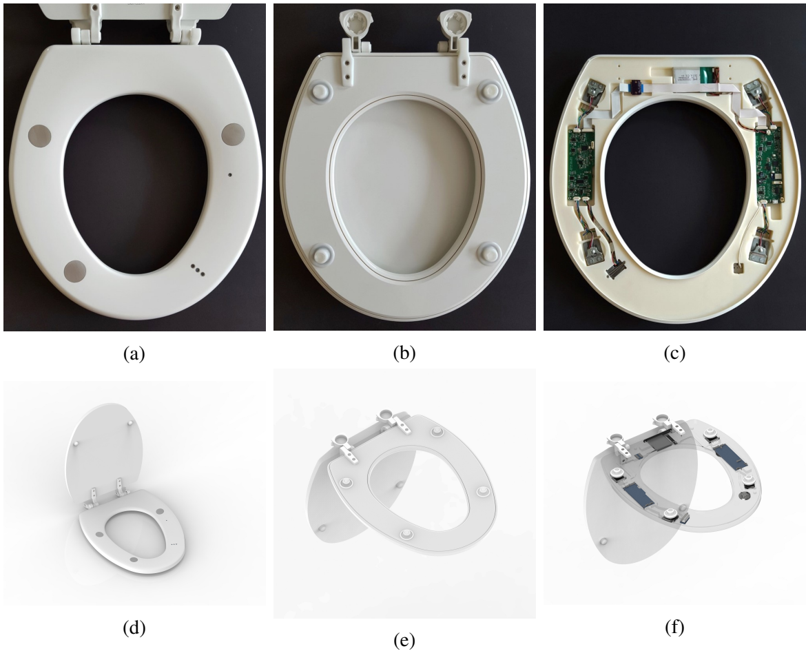
Figure 3.29: The in-hospital integrated version of the FIT seat is self-contained with all electronics and sensors inside of the seat. The seat is cleanable and the surface has no rough edges or crevices. Images of a completed seat and the 3D CAD renderings are shown (courtesy of Think Design).
