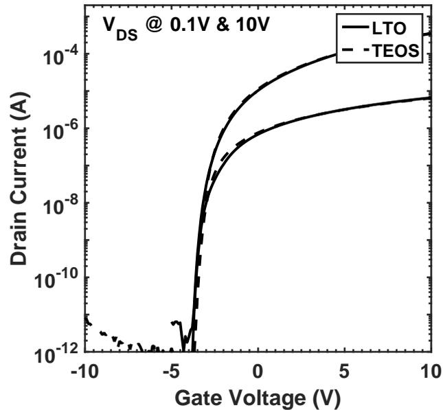
**Figure 4.8:** Transfer characteristics of TG<sub>stg</sub> TFTs with dimensions of  $L/W = 12/100 \mu\text{m}$ .
