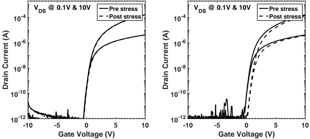
Figure 4.17: DG NBST (left) and PBST (right).
