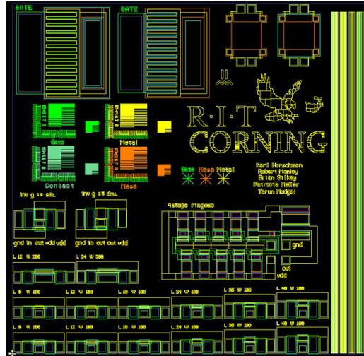
Figure 3.2: RIT TFT test chip layout.
