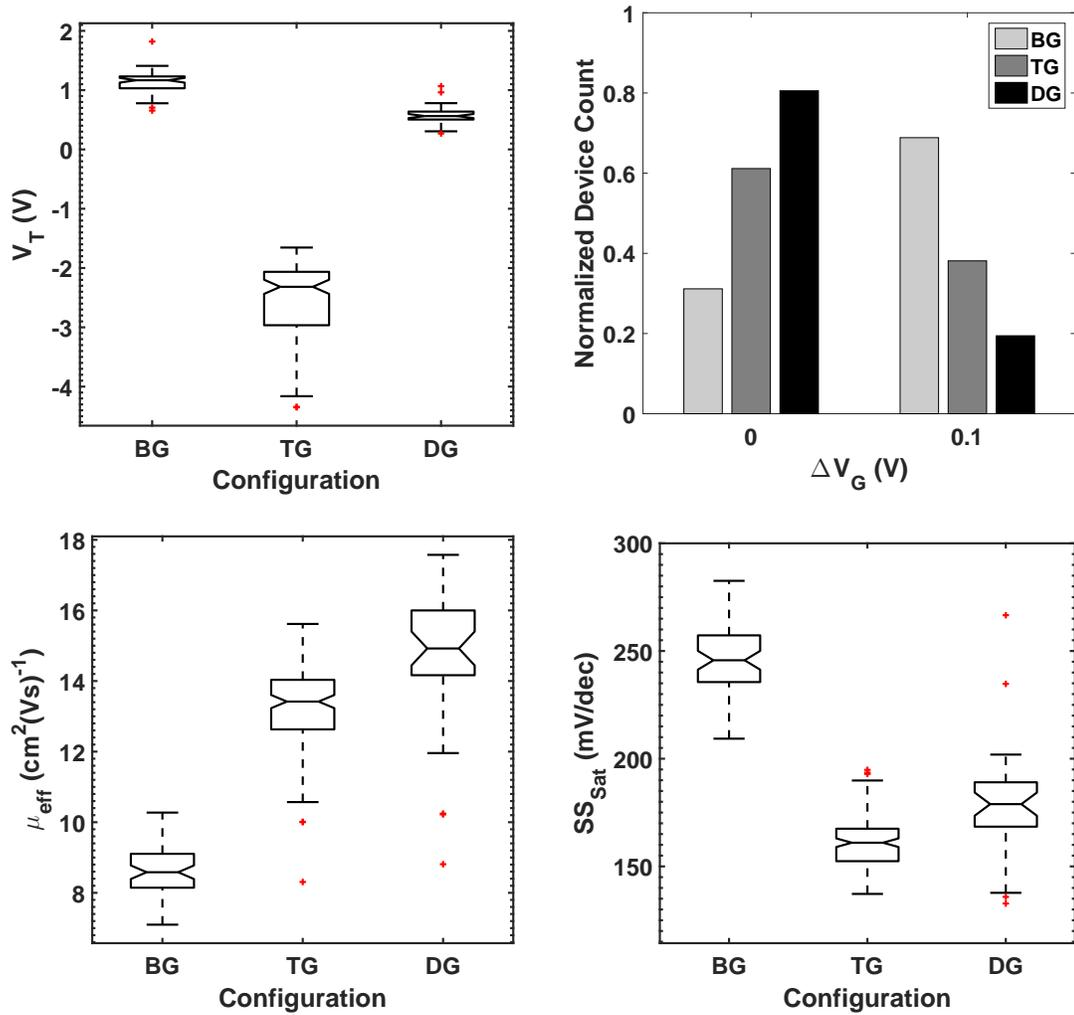
**Figure 4.14:** Extracted parameters from  $L/W = 12/100 \mu\text{m}$  devices with PECVD TG dielectric and 4 h anneals<sup>2</sup>.
