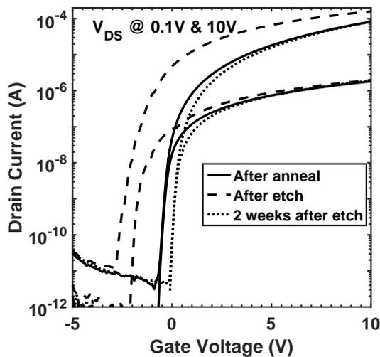
**Figure 3.6:**  $I_D - V_{GS}$  transfer characteristics of an  $L/W = 24/100 \mu\text{m}$  TFT after; annealing, wet etching the IGZO channel and 2 weeks after etching.
