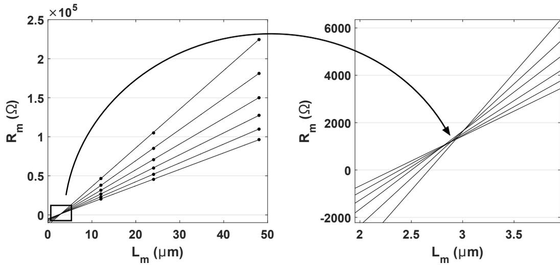
Figure 3.9: Terada-Muta analysis of IGZO TFTs.
