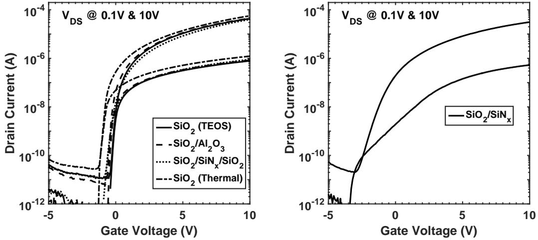
**Figure 3.4:** Overlay of PECVD and thermal  $\text{SiO}_2$  and ALD  $\text{Al}_2\text{O}_3$  transfer characteristics (left) and LPCVD  $\text{Si}_3\text{N}_4$  transfer characteristics with  $L/W = 48/100 \mu\text{m}$ .
