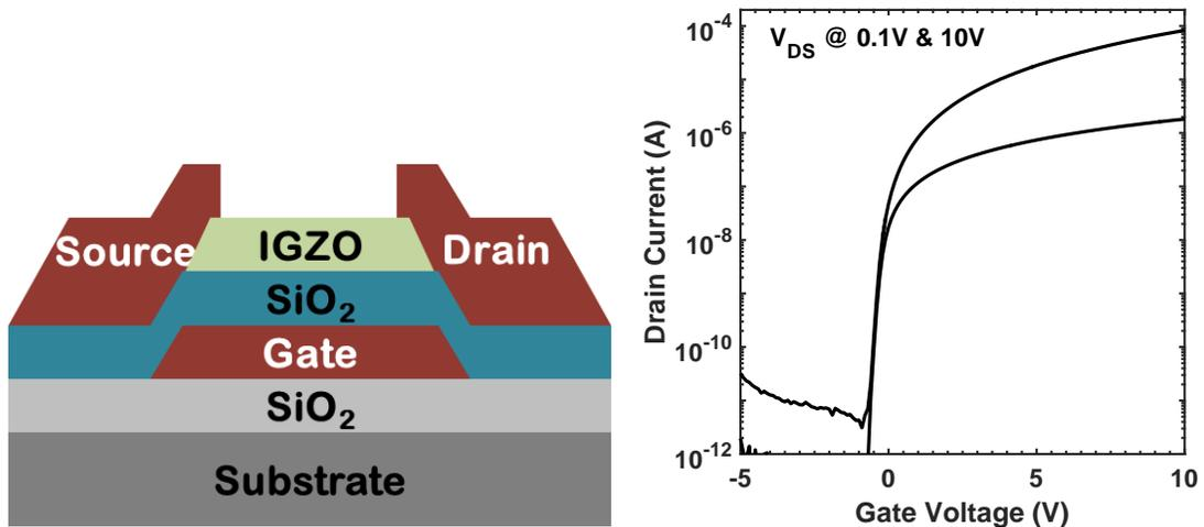
Figure 3.3: Structure of a BG<sub>stg</sub> IGZO TFTs without a back-channel passivation material (left) and the  $I_D - V_{GS}$  transfer characteristics of a L/W = 48/100  $\mu\text{m}$  TFT with  $V_{DS} = 0.1\text{ V}$  and 10 V [4].
