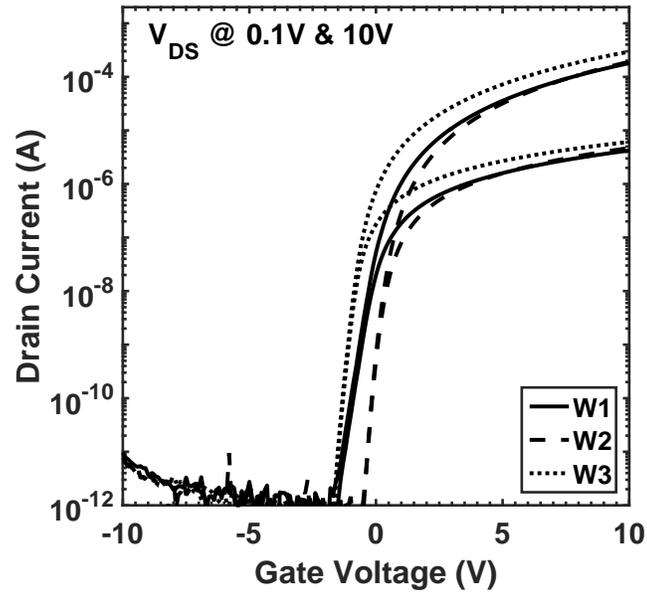
Figure 4.11:  $I_D$ - $V_{GS}$  transfer characteristics of DG TFTs.
