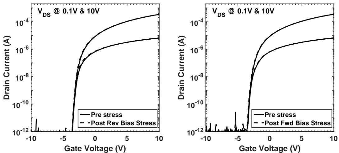
Figure 4.16:  $\text{TG}_{\text{stg}}$  NBST (left) and PBST (right).
