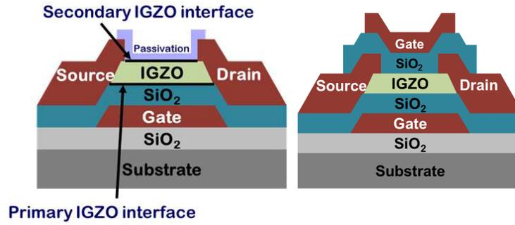
**Figure 4.10:** Cross-sectional image comparing BG<sub>stg</sub> (left) and DG (right) TFT structures.
