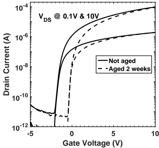
**Figure 3.5:** Transfer characteristics of an  $L/W = 24/100 \mu\text{m}$  TFT immediately after annealing and 2 weeks after annealing.
