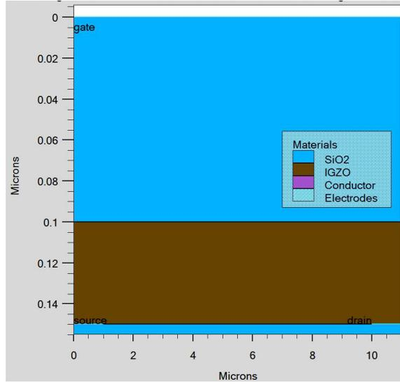
**Figure 5.1:** Simulated structure of a  $TG_{stg}$  TFT where  $L_{eff} = 9 \mu\text{m}$ .
