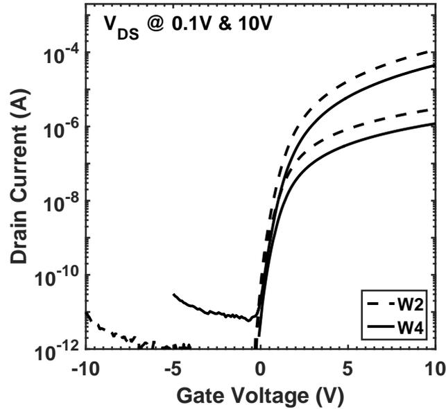
**Figure 4.3:**  $I_D$ - $V_{GS}$  transfer characteristics of over-oxidized IGZO L/W = 12/100  $\mu\text{m}$  SiO<sub>2</sub> passivated TFT.
