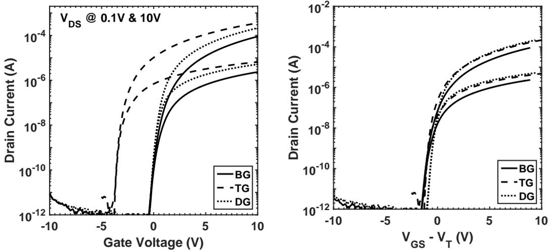
**Figure 4.13:**  $I_D$ - $V_{GS}$  transfer characteristics of BG, TG<sub>stg</sub> and DG configurations with dimensions of  $L/W = 12/100 \mu\text{m}$  as measured (left) and normalized x-axis (right).
