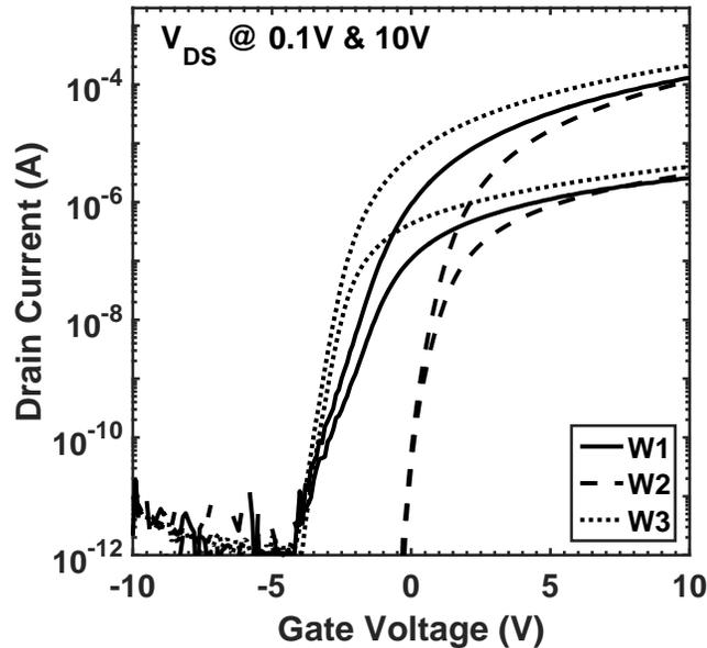
**Figure 4.2:** BG  $I_D$ - $V_{GS}$  transfer characteristics of  $L/W = 12/100 \mu\text{m}$  SiO<sub>2</sub> passivated TFTs.
