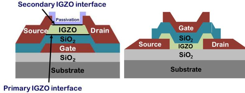
**Figure 4.7:** Cross-sectional image comparing BG<sub>stg</sub> (left) and TG<sub>stg</sub> (right) TFT structures.
