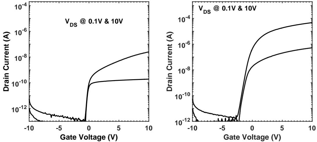
**Figure 4.6:** TG<sub>cop</sub>  $I_D$ - $V_{GS}$  transfer characteristics with  $L/W = 12/100 \mu\text{m}$  of wafer 1 (left) and wafer 3 (right).
