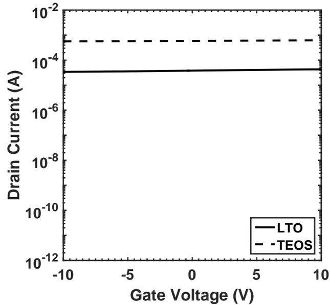
**Figure 4.1:**  $I_D$ - $V_{GS}$  transfer characteristics of SiO<sub>2</sub> passivated TFTs,  $V_{DS} = 10$  V.
