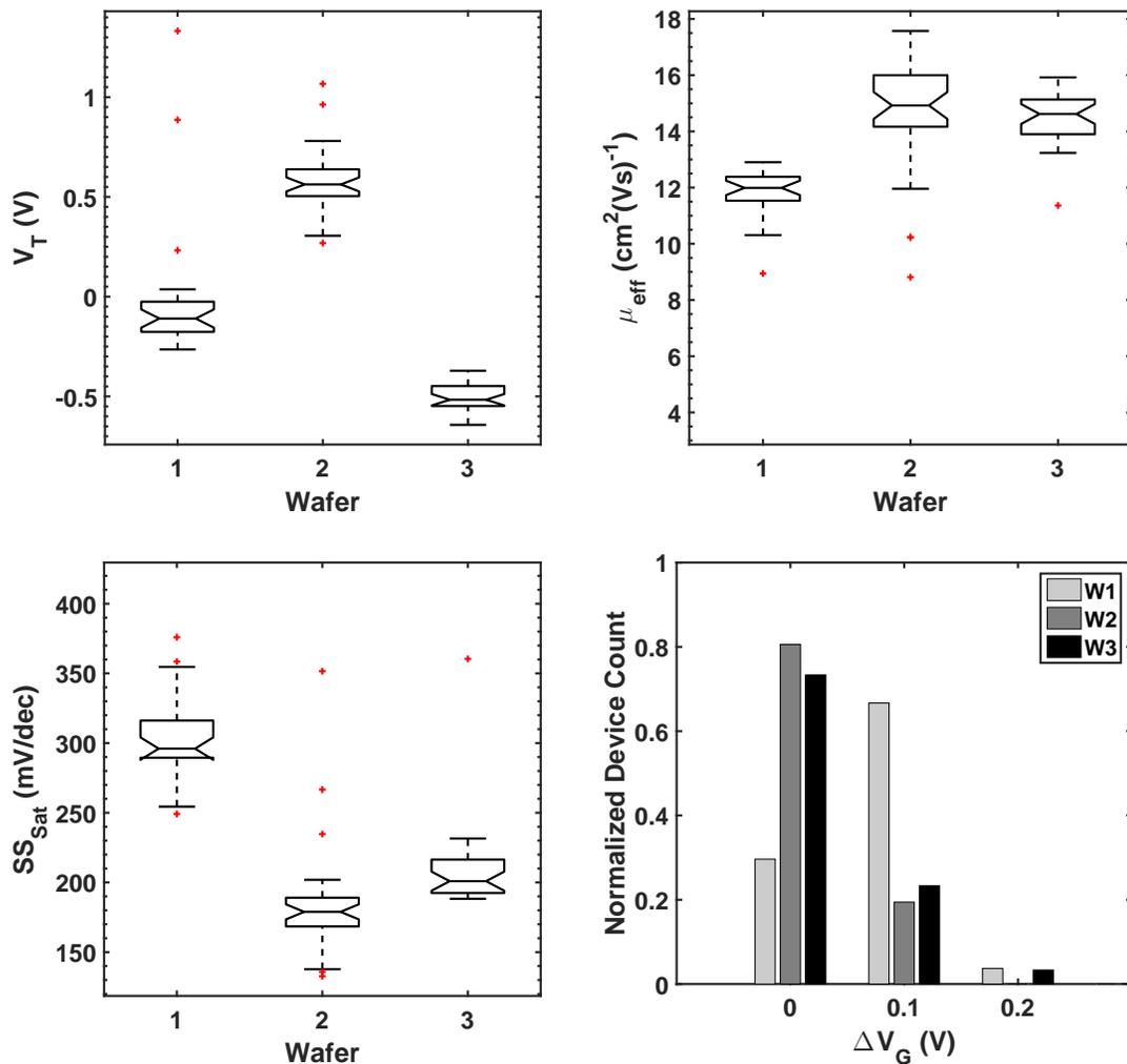
**Figure 4.12:** Box plots of extracted parameters for  $L/W = 12/100 \mu\text{m}$  DG configuration wafers 1 – 3.
