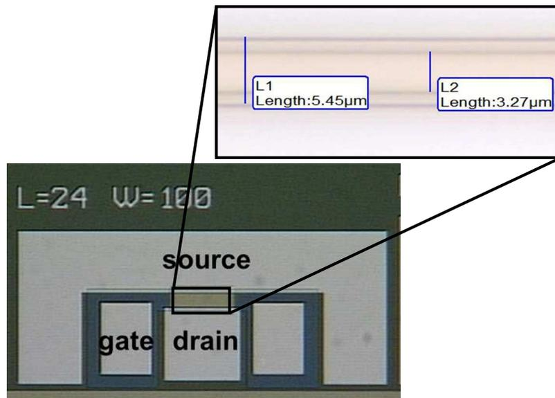
Figure 3.10: S/D lift-off lithography bias with a mask defined channel length of 6 μm.
