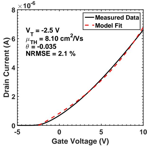
Figure 2.3: Measured and modeled  $I_D$ - $V_{GS}$  transfer characteristics.
