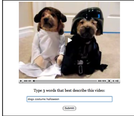
Figure 1: A video CAPTCHA. A challenge is passed if one of the three tags submitted by a user belongs to an automatically generated set of ground truth tags. Online demonstration: http://sudbury.cs.rit.edu/
