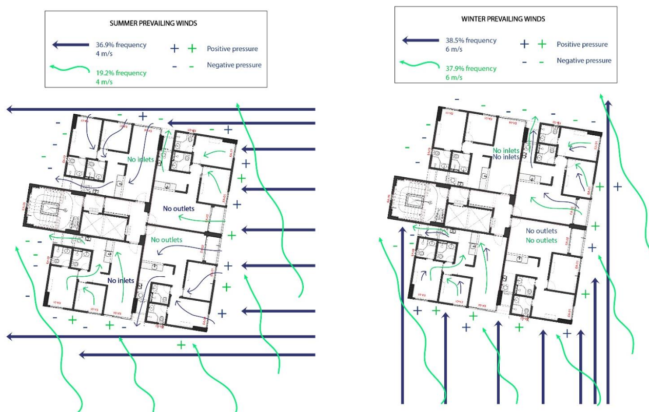
Figure 52 - Winds incidence in a typical floor on the baseline building representing summer conditions(left) and winter conditions (right).
