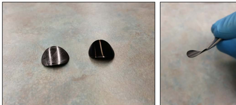
Figure S14: CNT array devices after cleaning in high temperature furnace at 700 °C for 4 hours, indicating the curled devices.
