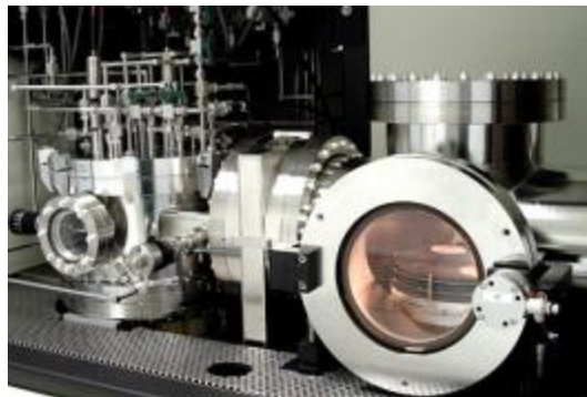
Figure 2.8. Image of the MOCVD reactor at the NASA Glenn Research Center.
