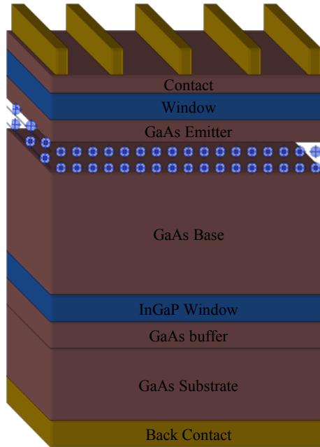
Figure 2.9. Cross section of GaAs single junction solar cell embedded with QDs.
