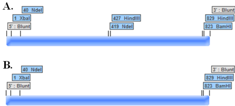
Figure 7. Predicted restriction sites for wildtype gene and synthetic gene. (a. wild type b. synthetic gene) Restriction sites are shown for BamHI, HindIII, NdeI, and XbaI enzymes.
