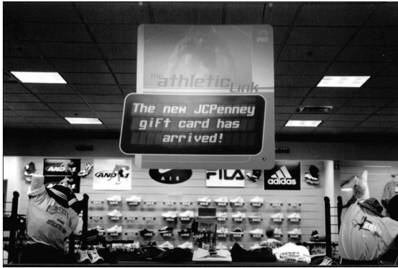
Figure 22. The first commercial use of E Ink technology was in May 1999 in the J.C. Penney Athletic Link department in their Marlborough, MA store. The content of the sign could be changed by the store manager through a wireless link. The three month trial was part of a field experiment involving over 30 retailers. Results of the trials led to the development of the second-generation sign product: Ink-In-Motion. (Photo courtesy of E Ink)
