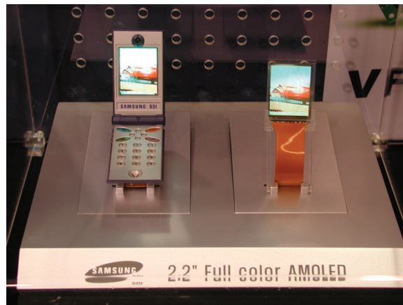
Figure 30. With the inclusion of an OLED display, this Samsung cell phone will operate for much longer than it would using an LCD. (Photo by author)
