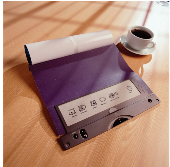
Figure 11. The flexible "eNewspaper" backplane contains a touch-sensitive control panel used to manipulate its content. (Photo courtesy of the IBM Strategic Design Group)
