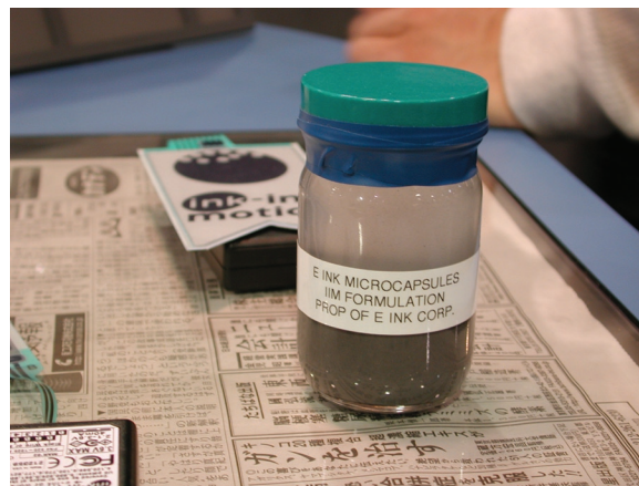
Figure 21. A jar containing the E Ink particles. Close examination shows that the particles have separated from the light oil carrier. (Photo by author)
