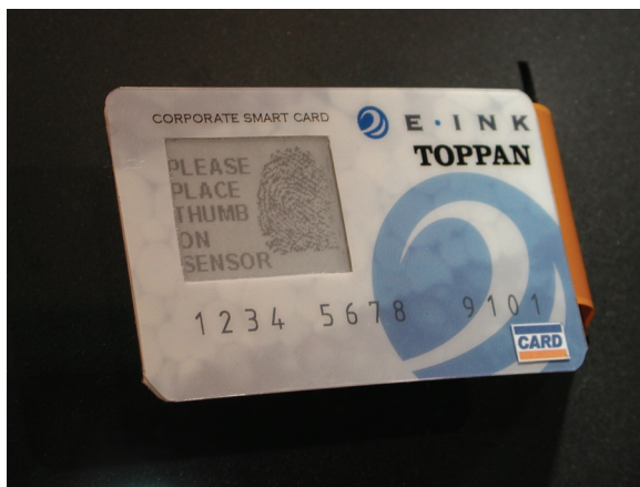
Figure 19. A prototype for a smart card containing an E Ink display. (Photo by author)
