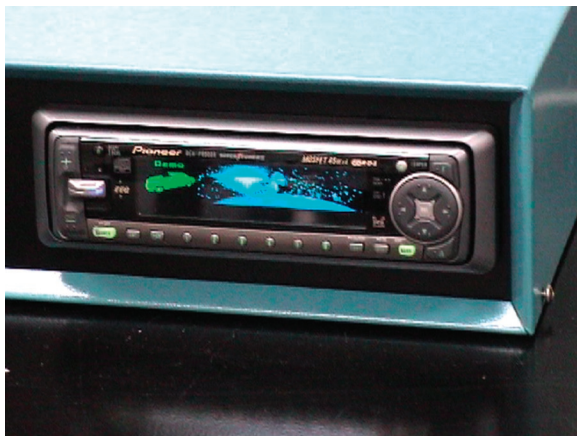
Figure 32. This Pioneer radio faceplate is the first to use OLED as a component in a commercial product. (Photo by author)
