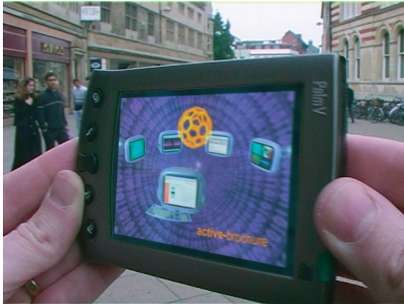
Figure 34. Improved screen displays, such as this prototype CDT color display built into a Palm V PDA, provide the means to read the screen under any lighting conditions and at any angle. (Photo courtesy of Cambridge Display Technology)
