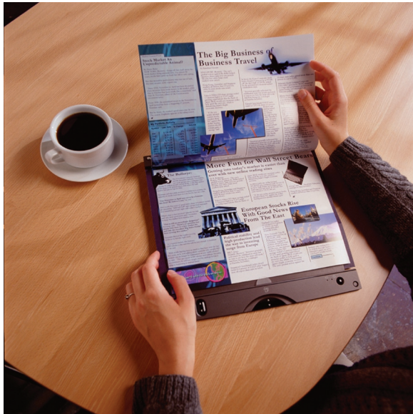
Figure 10. Flexible pages will compose a section of the IBM eNewspaper. These pages are reimageable to display successive sections comprising one or more issues of the newspaper. (Photo courtesy of the IBM Strategic Design Group)
