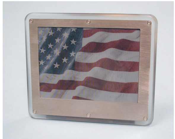
Figure 25. The first high-resolution, active-matrix color display made with electronic ink measures 5 inches diagonally, with a resolution of 320 x RGB x 234 (80 ppi). It is constructed of components from each of its co-developers: the electronic ink layer from E Ink, the color filter arrays from TOPPAN Printing, Ltd., and the active matrix backplane from Philips. The display was announced on July 1, 2002. (Photo courtesy of E Ink)
