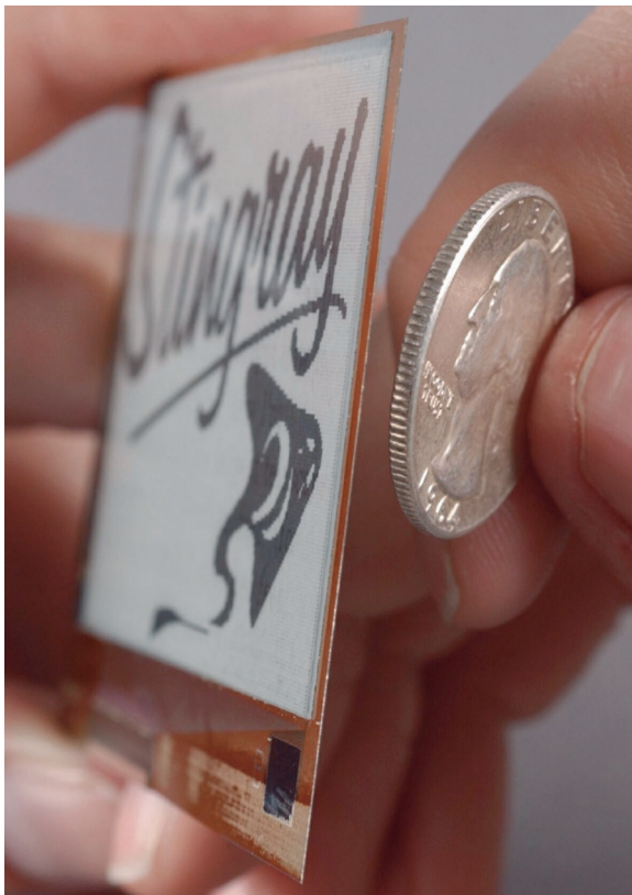
Figure 28. E Ink's prototype display, expected to be in wide distribution by 2004-2005, is the world's thinnest active matrix display with a thickness of 0.3 mm. (Photo courtesy of E Ink Inc.)
