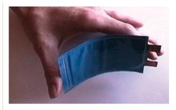
Figure 24. A prototype of the MIT battery. (Photo courtesy of VoltaFlex)
