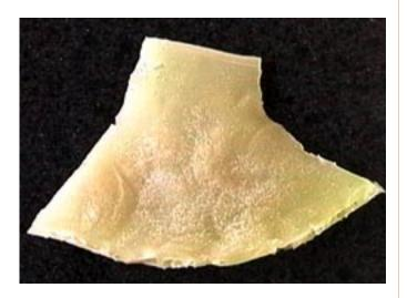
Figure 23. A sample of the polymer invented at MIT which is used in the VoltaFlex batteries. (*Photo courtesy of VoltaFlex*)
