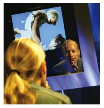
Figure 13. The Mirror TV appears as a normal mirror when the display is not on. It provides the benefits of hiding the TV from sight as well as making the room or workspace appear larger. Philips anticipates that the display will be popular in hotels which need to conserve space as much as possible.
