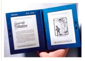
Figure 6. This prototype double-page e-reader, combining an E Ink display and Philips TFT backplane, is the first commercial product resulting from the E Ink and Philips partnership. (Photo courtesy of Philips. Used with permission.)
