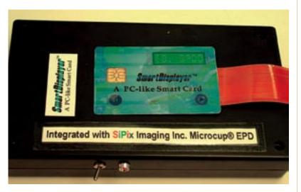
Figure 19. A small Microcup display fabricated in a smart card prototype. (Photo courtesy of SiPix)
