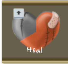
Figure 5.20 - Radial fill being used to indicate the cooldown of an ability. The math is part of the shader that render sprites.
