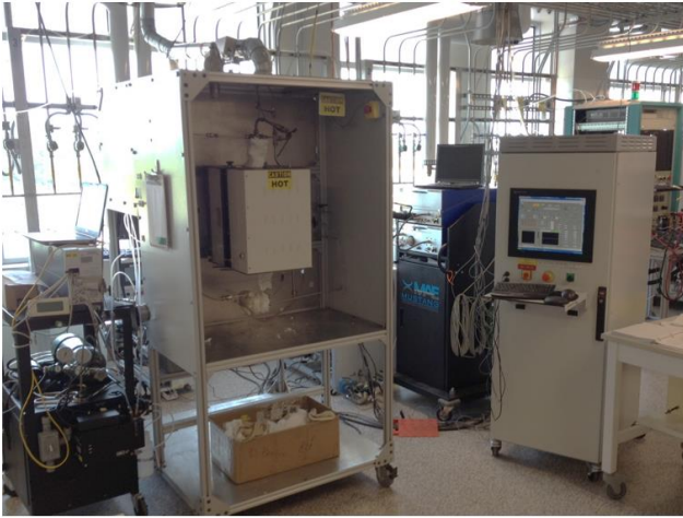
Figure 10: Left fuel reformer facility with associated instrumentation, right: propane cPOx test cell schematic containing Inconel single tube reactor based on Microlith (catalytically coated meshes) catalyst technology (31.75 mm diameter, 8.9 mm length).
