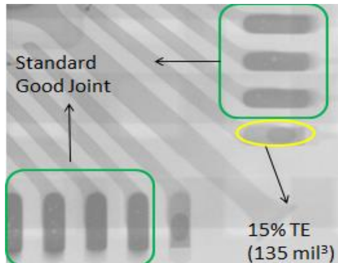
Figure 54 X-ray image of QFN 100 on Cu-OSP with a functional solder joint with 15% TE (135 mil 3 ).
