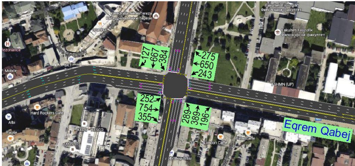
Figure 9: Intersection Design and Inputs in Synchro 8.0
