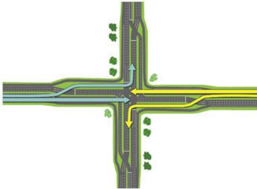
Figure 6: Continuous Flow Intersection (Lee, 2013)
