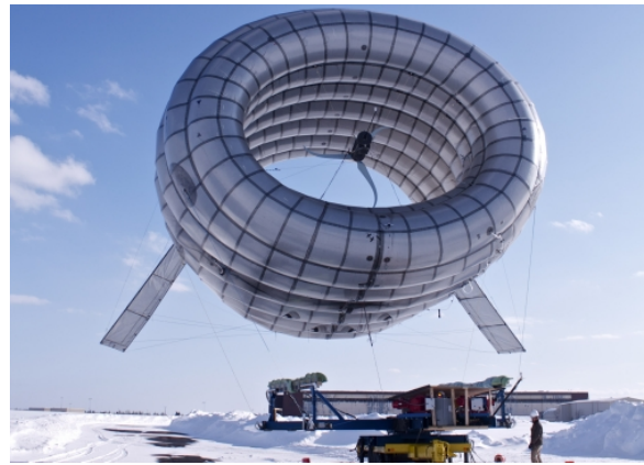
Fig. 1.11: Altaeros Energies 35ft Diameter Prototype [3]
