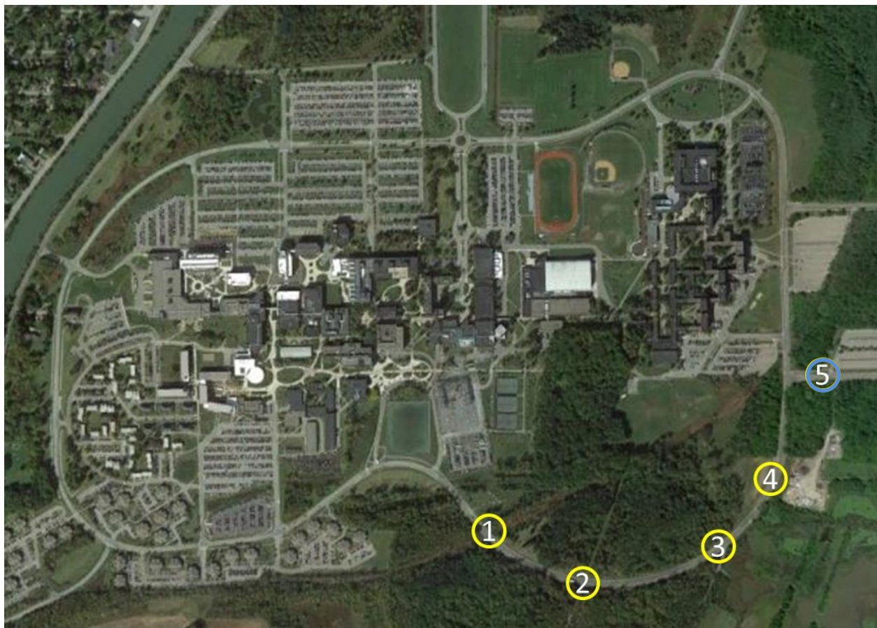
Figure 25: An aerial image of RIT with recommended locations of speed bumps circled in yellow.
