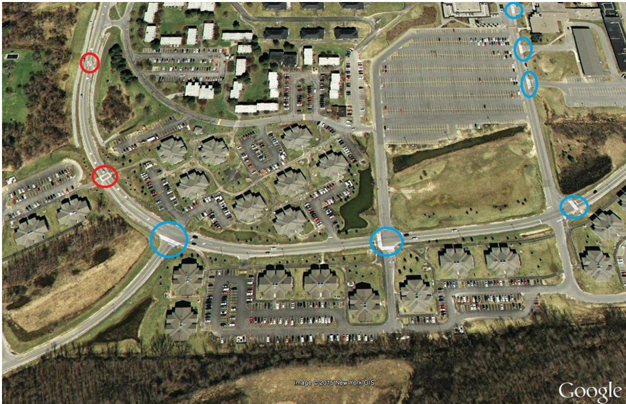
Figure 18: An aerial image of the University Commons complex in the southwest section of campus in 2006. Red circles indicate speed bumps and raised crosswalks, while blue circles indicate painted crosswalks.
