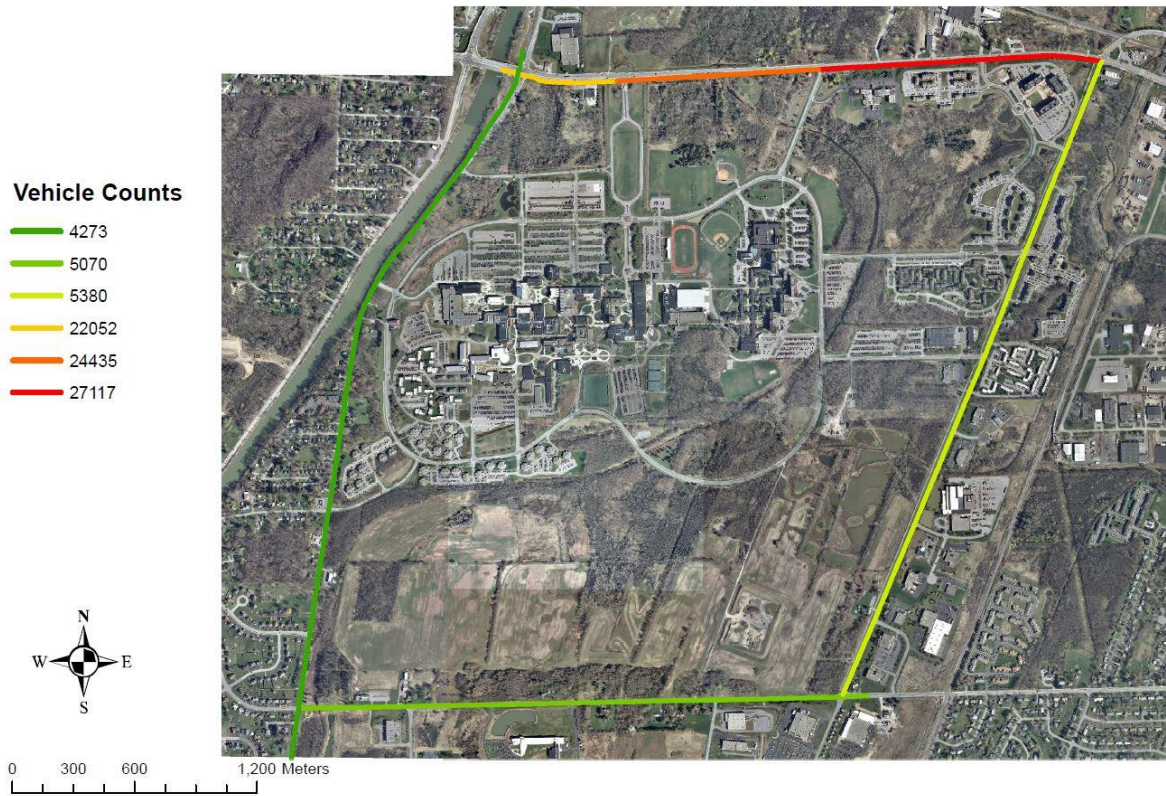
Figure 9: Daily vehicle counts based on data from the New York Department of Transportation. The data are based on 2013 counts.
