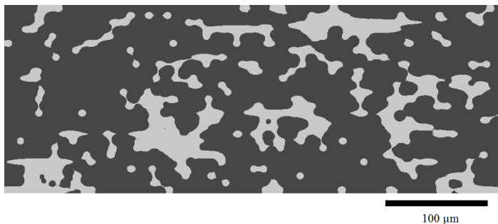
Figure 3.34: Simulated Toray TGP-H-060 with 0 wt.% PTFE showing the fiber and binder distributions similar to an actual GDL shown in Fig. 3.33(b).
