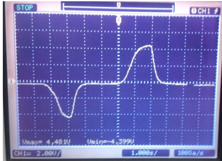
Figure 16: Sensor output showing V_{max} and V_{min} of the hall device in the presence of +6275 G and -6275 G magnetic fields.
