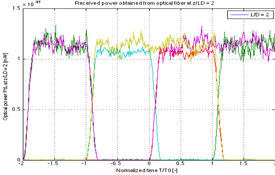
Figure 7.8: Received signal P_{dc}(0, T) from an optical fiber at \frac{z}{L_D} = 2 and resolution = 6
