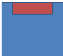
Figure 2.5: Cartoon of the PEDOT:PSS coated ITO (blue) with Kapton tape affixed on top (red rectangle). The tape is removed when testing the devices to expose the ITO contact.
