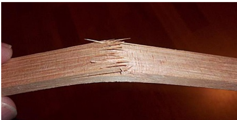
Figure 3.11.4 Failure in bending
