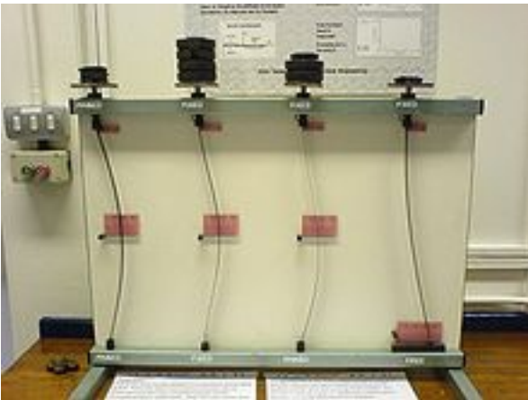
Figure 3.12.3 Types of buckling deformation (Wikipedia)
