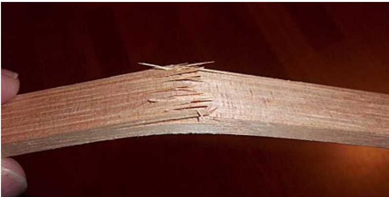
Figure 3.9.3 Failure in bending (The following images are obtained from Wikimedia commons)
