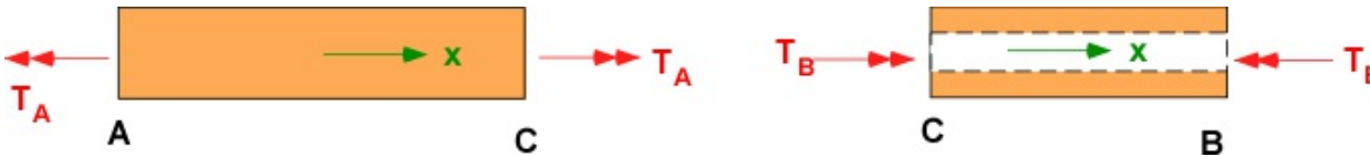
Figure 8.2.3c. FBD of parts of shaft
