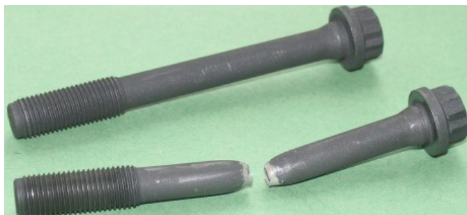
Figure 3.9.1 Failure in tension (necking)
