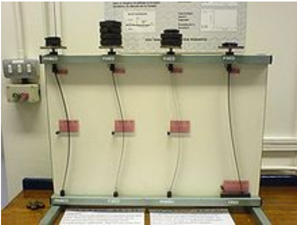
Figure 9.1.1 Types of buckling deformation (Wikipedia)
