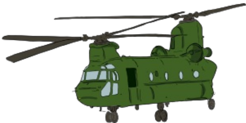
Figure 2.1.2 Contra-rotating rotors providing action and reaction
